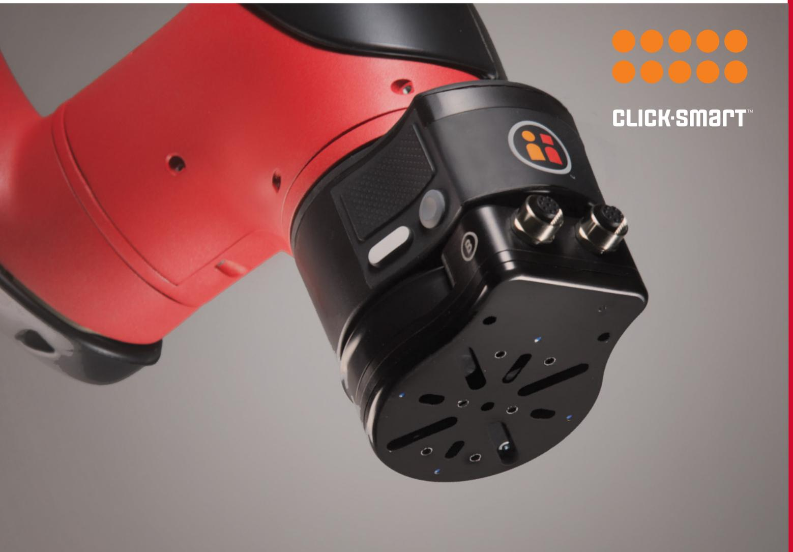
The ClickSmart Plate is the cornerstone of the ClickSmart family – its quick release mechanism enables rapid changing of End of Arm Tooling (EOAT) in seconds, without using any tools. The ClickSmart Plate has an embedded memory module, which stores the configuration of the attached EOAT. When the ClickSmart Plate is attached to any Sawyer robot, it will immediately recognize the type of end-effector and know how to control it. A simple click solves the problem!
